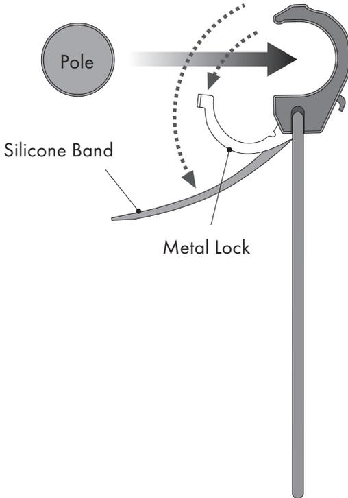
Be sure to open the metal lock before removing.
