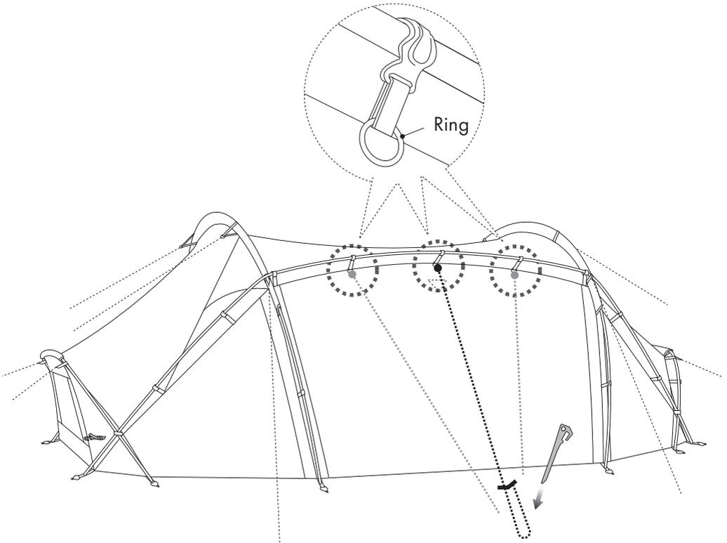
Attach a rope to the center point
